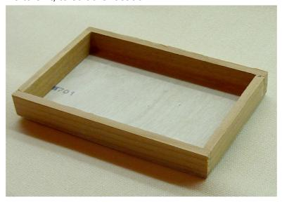
I made the box 80mm wide only because that was the gap between the ribs. It could be made a lot narrower to suit the servo and model. The lid has a strip of 1mm birch ply around the edges of its underside and squares in the corners. These allow a little more thickness for countersinks for the M2 x 4 screws holding it down.
