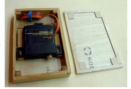
This shows the servo in position. 5mm square spruce was exactly the correct size to form the frame into which the servo fits. Short 2mm servo screws hold the servo down.
