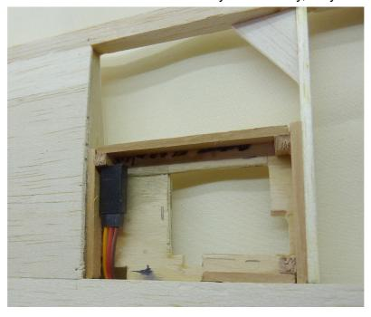
So I decided to design a mounting box for future versions and other models. The boxes will be installed when fitting ribs rather than at the end.
