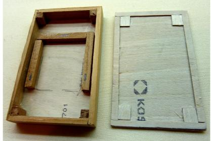
This shows the box with the servo frame and corner blocks glued in.
