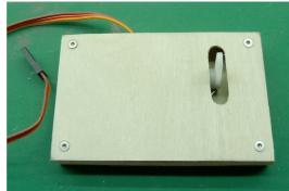
Total weight without the servo is 11.4g. I will probably do away with connectors to save space and weight by soldering the leads and using heat shrink. I am also testing two other slim wing servos from Hobby King, the HK15322MG (£7.61 1.75 kgcm digital) and the Turnigy BMS-555MG (£16.36 4.2 kgcm analogue).
